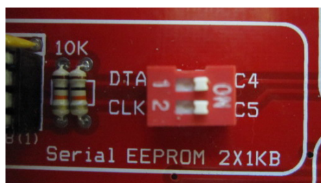
Figure 53. Enable serial EEPROM (24Cxx)
