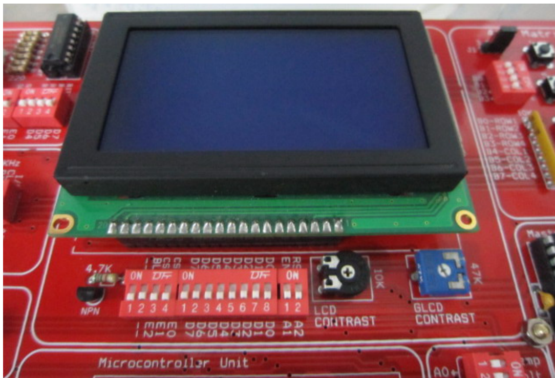
Figure 23. 128X64 GLCD display unit real PCB view.
